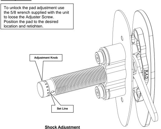
To adjust the resistances of the hydraulic shock absorber, or to remove the system from the stock, follow these steps.
